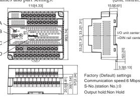
Changes termination ON/OFF. Turns ON only A: Terminal Switch the unit connected at the end of the communica tion cable
