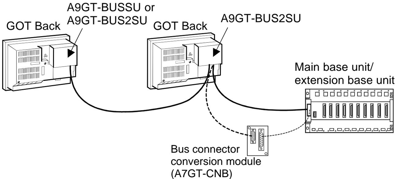
With the A9GT-BUS2SU, the dimensions of the cable that protrudes from the bottom of the GOT are smaller than the A9GT-BUSS/A9GT-BUS2S type bus connection interface board (hereinafter, bus connection board) used with the conventional bus connection.
