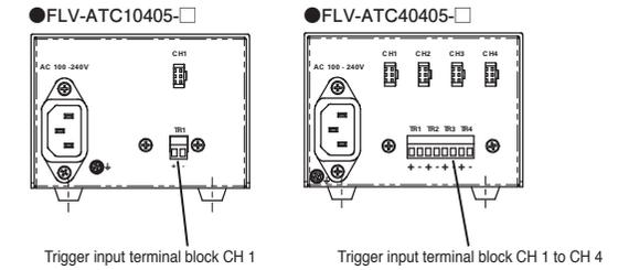
Short-circuiting (+) and (-) of TR1 to TR4 respectively makes the trigger input status OFF, turning the light OFF.
