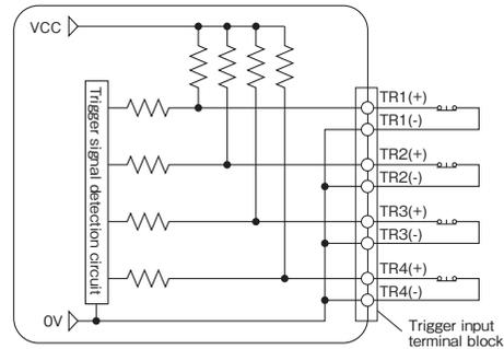
※Current flowing through the short circuit is less than 1mA.
