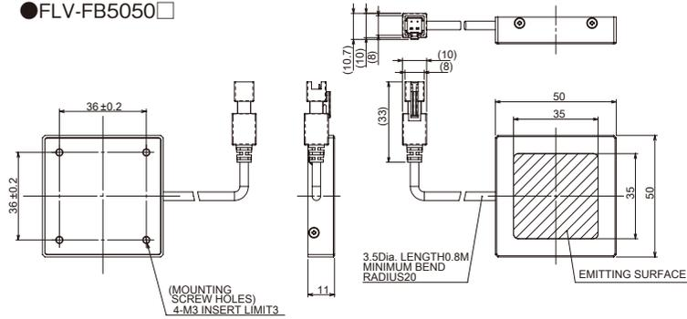
Tightening torque:  $0.54N \cdot m$
