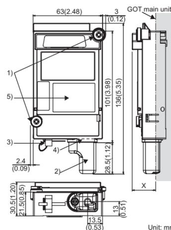
\* The external dimensions of printer unit with a cable clamp and connector holder attached is shown above.
