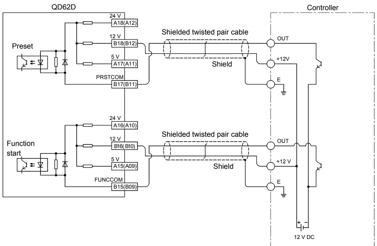
When the controller (source loading type) is 5 V DC:
