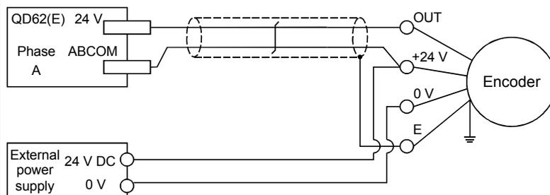
[Incorrect wiring example]
