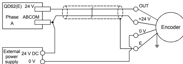
The current flows through the shielded twisted pair cable in the same direction, so there is no cancelling effect. This makes it more prone to electromagnetic induction.
