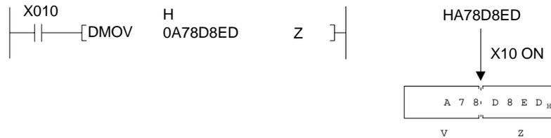
If either of Z or V is specified for index qualification in the instruction, index qualification is performed regarding data in Z and V as 16-bit data even when 32-bit data is stored in Z and V.
