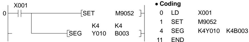
(2) Pulse output using the SET and RST instructions in direct mode should be changed as shown below when the I/O control is changed to refresh mode.
