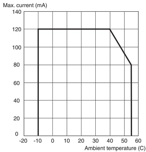
\* The value for standard mounting. Be careful because the derating curve differs depending on the mounting.
