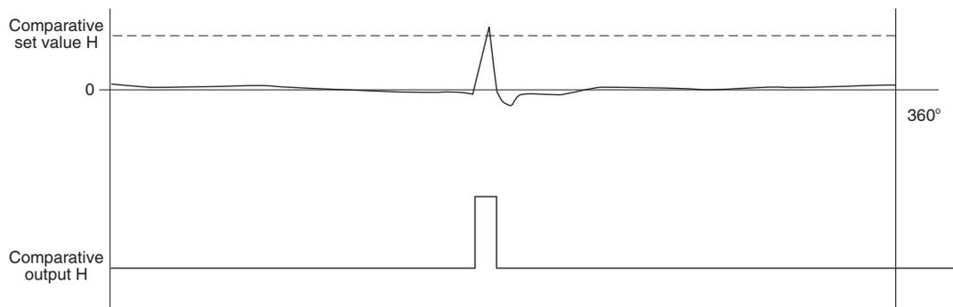
Previous average comparison makes the measurement value the difference between the present input value and the average of all previous input values.
