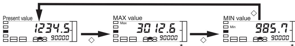
\* If the operation at input error (*S.Err*) is set to *S.Err* and if a sensor error occurs, *R.Err* or *b.Err* is held by the maximum and minimum values.
