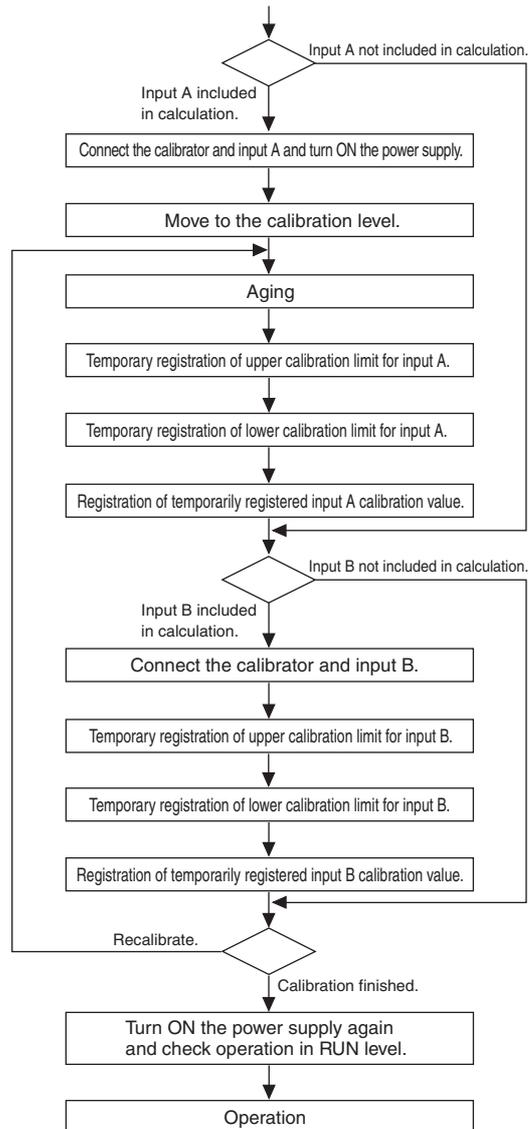
The input type that can be calibrated according to this flowchart is the type selected under "input type A" or "input type B".
