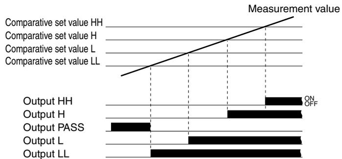
\* PASS output turns ON when any HH, H, L, or LL outputs turn OFF.
