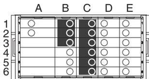
The sensor power can be supplied from terminals B5 and B6. The power supply specifications are outlined below.
