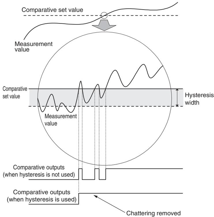
Hysteresis works in direction of decreasing measurement values for comparative set values HH and H and works in the increasing measurement value direction for comparative set values LL and L.
