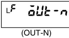
The comparative output logic for comparative results is set using the following parameter.
