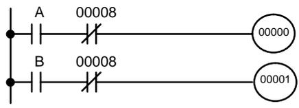
Since alarm output bit 08 covers both output bits 00 and 01, both these outputs are forced OFF as soon as output bit 08 turns ON (bits A and B can be any other bits required in the program).
