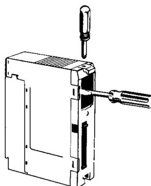
6. Pull out the printed circuit board.
