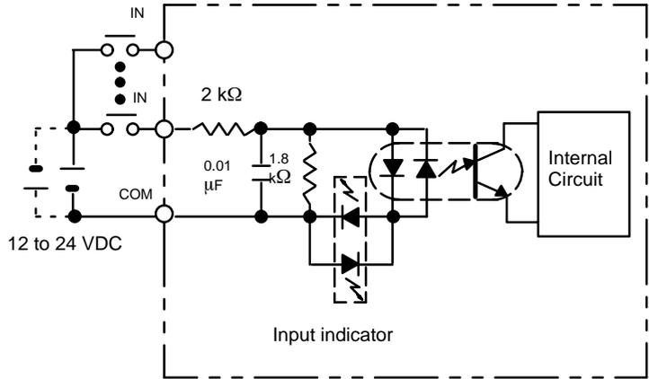
Either plus or minus can be used for the input power supply.
