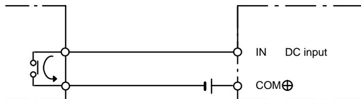
When using the NPN-current-output configuration shown below, the sensor and Input Unit should receive their power from the same supply.
