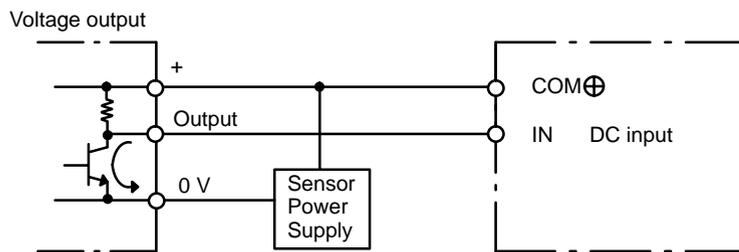
The circuit below should **NOT** be used for I/O devices having a voltage output.
