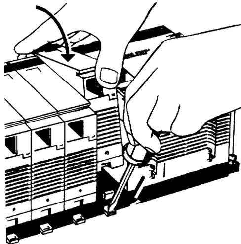
(To remove a Unit, hold down the lock lever with an implement such as a screwdriver.)
