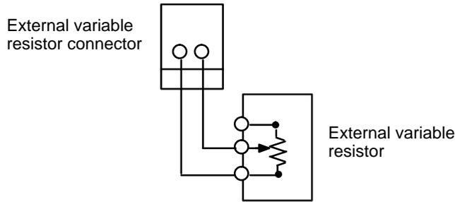
**Caution** Ensure that the external variable resistor connectors are open when using the internal variable resistor.
