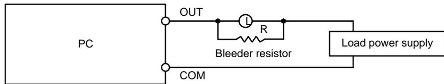
Determine the value and rating for the bleeder resistor using the following formula.
