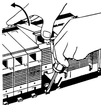
4. Using a Phillips screwdriver, remove the screw from the top of the Unit.
