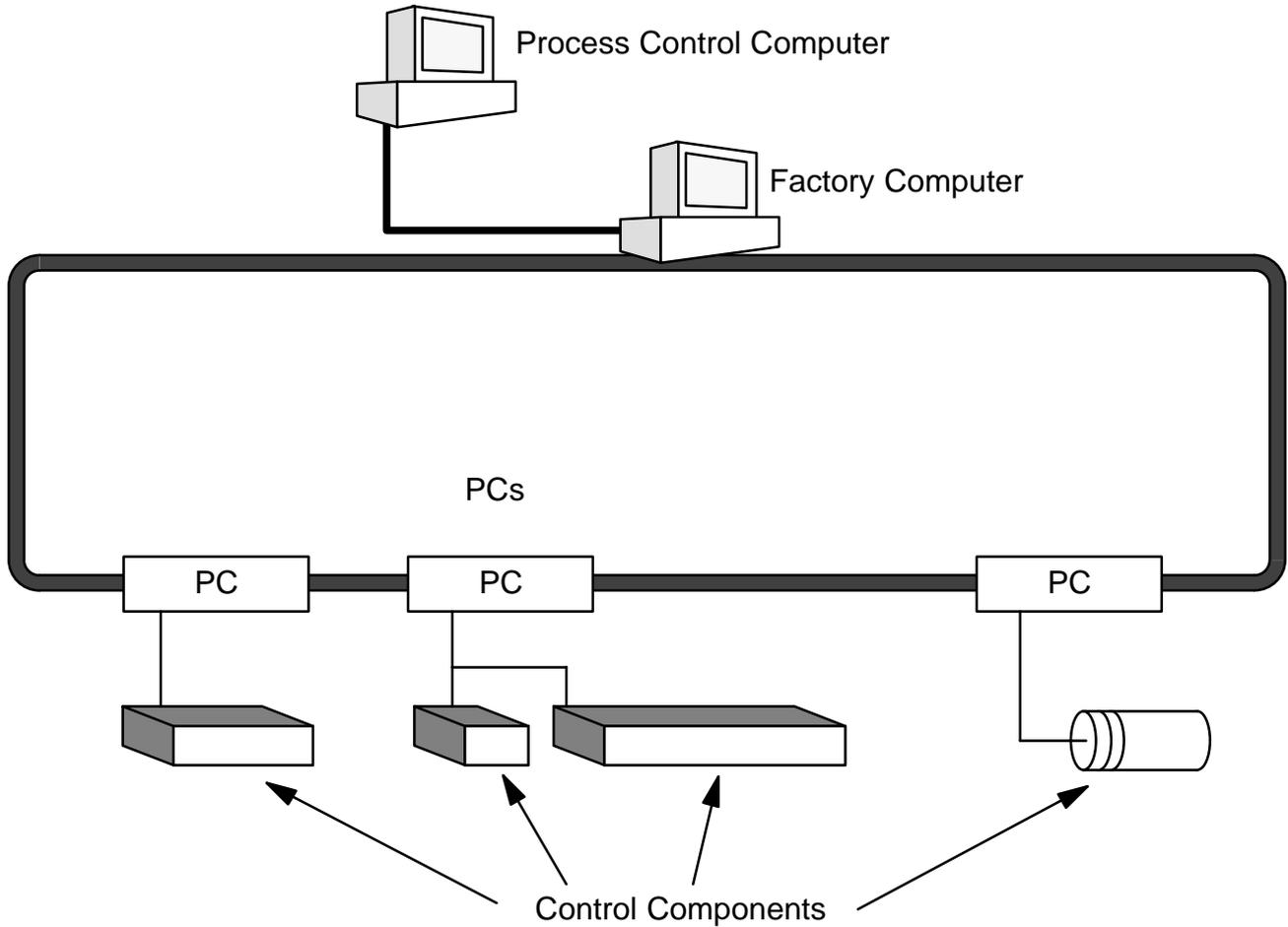
A Control System can involve very large applications where many different models of PC are networked together or it could be an application as small as a single PC controlling a single output device.
