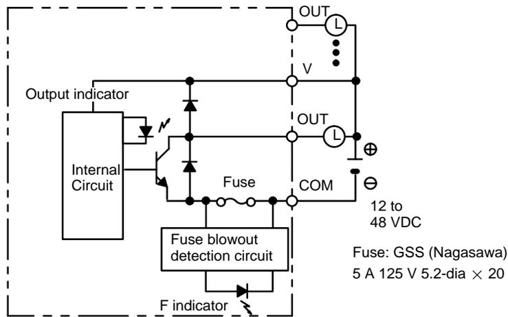
**Note** When the fuse blows, the F indicator lights and bit 08 turns ON. Bits 08 through 15 cannot be used as IR bits.
