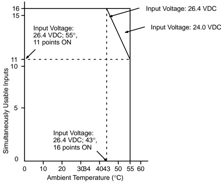
**Note** If the Unit is at room temperature it takes about 10 minutes for excessive heat to build up when all inputs are turned ON, so all inputs can be turned ON simultaneously for testing.
