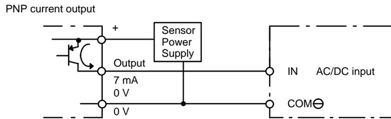
The circuit below should be used for I/O devices having a voltage output.
