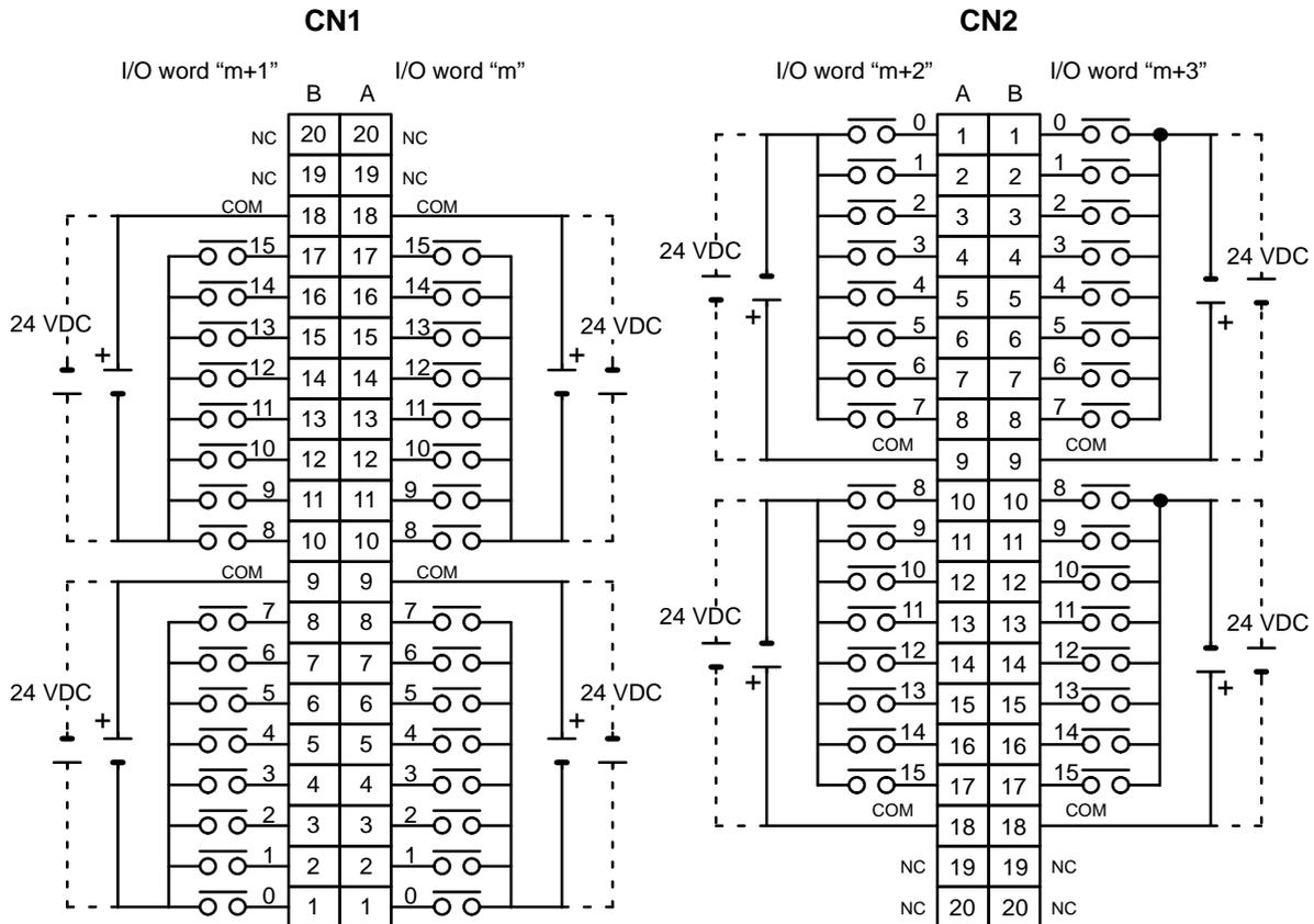
**Note** 1. I/O word “m” is determined by the I/O number setting ( $m = IR\ 030 + 2 \times \text{I/O number}$ ).
