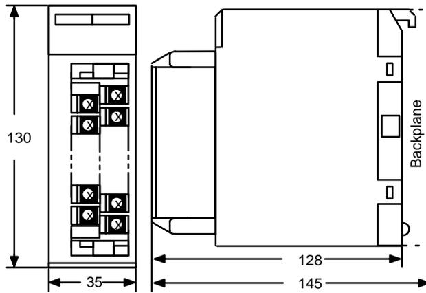
**10-terminal Terminal Block (E-shape I/O Units)**
