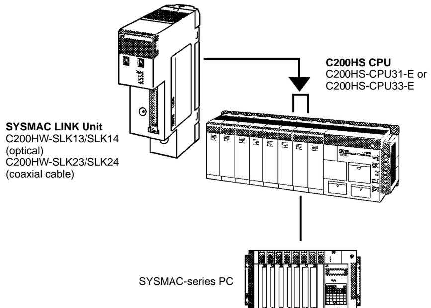
**SYSMAC NET Link Systems** OMRON's SYSMAC NET Link System is an FA-oriented limited-area network that connects up to 126 nodes to provide datagram services, data transfers, and data links.
