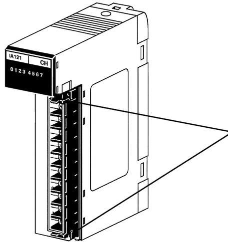
Locks for terminal block. Unlock to remove the terminal block from the I/O Unit. Make sure the terminal block is locked securely after wiring is complete.
