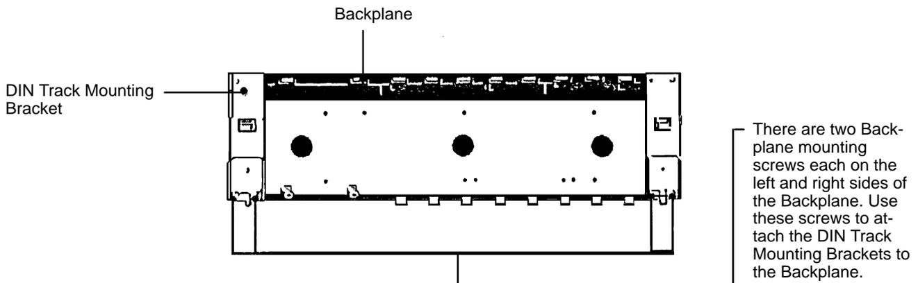
2. Mount the Backplane to the DIN Track so that the claws on the Mounting Brackets fit into the upper portion of the DIN Track as shown below.
