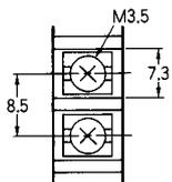
Use hook-type crimp connectors with a line thickness of 0.25 to 1.65 mm<sup>2</sup>. The construction of the terminals is shown in the illustration.
