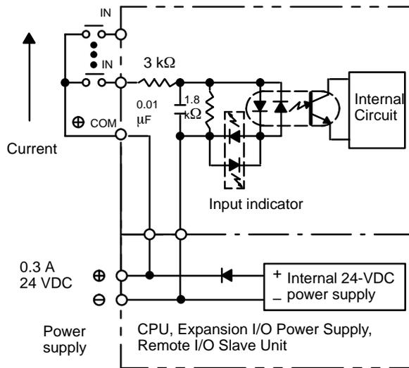
**Note** The power is supplied to the Input Units from the 24 VDC output of the Power Supply of the CPU, Expansion I/O Unit, or Remote I/O Unit. Never connect 24 VDC output terminals to the input terminals or COM terminals.
