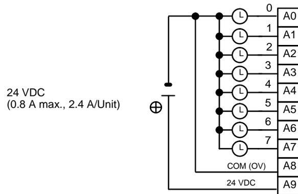
**Note** Be sure to supply power to A9; otherwise current will leak through the load while the output is OFF.
