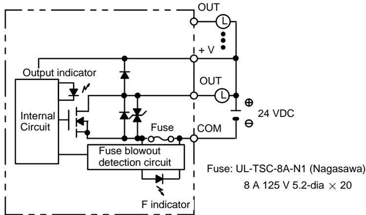
**Note** When the fuse blows, the F indicator lights and bit 08 turns ON. Bits 08 through 15 cannot be used as IR bits.
