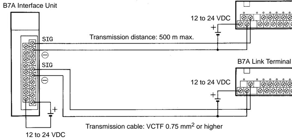
**High-speed Transmission Delays (3 ms): Shielded Cable**
