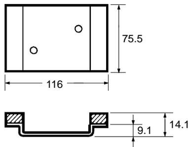
Take the space required for the cable into consideration when mounting the Programming Console to panels.
