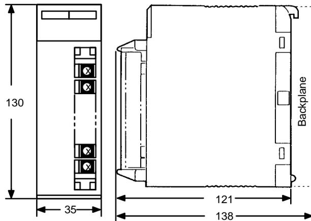
**19-terminal Terminal Block (Extended B-shape I/O Units)**
