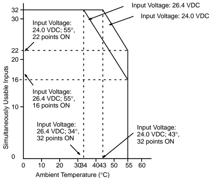
**Note** If the Unit is at room temperature it takes about 10 minutes for excessive heat to build up when all inputs are turned ON, so all inputs can be turned ON simultaneously for testing.
