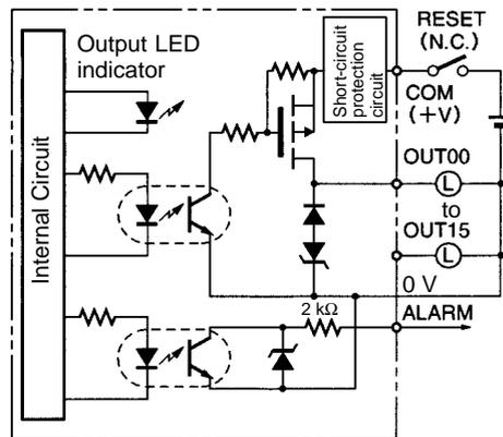
**Note** 1. When the short-circuit/overload protection is activated, all 16 outputs are switched OFF and the ALARM output becomes active (low level). It is possible to determine the cause of the alarm by connecting either a DC Input Unit to the alarm output or an alarm output LED indicator.
