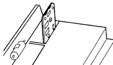
5. Replace the Memory Cassette bracket over the Cassette and tighten the screw that holds the bracket.
