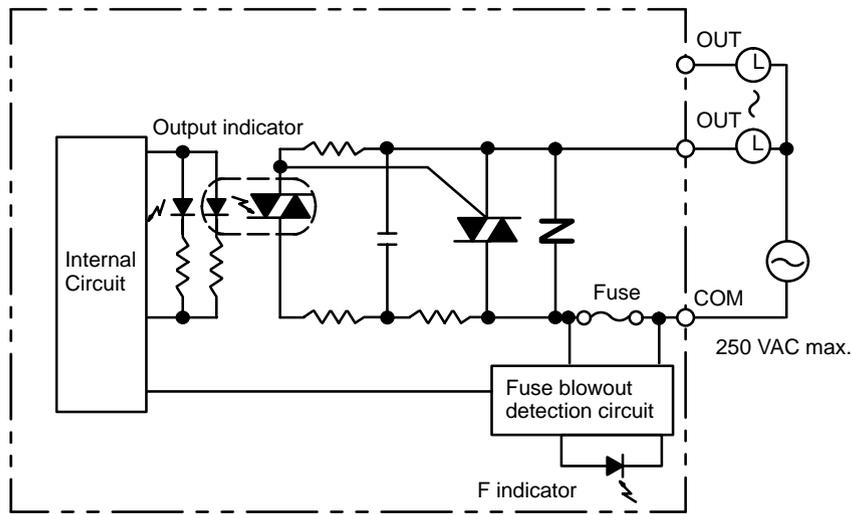
Fuse: 5 A 250 V (5.2-dia.x20) HT (SOC)
