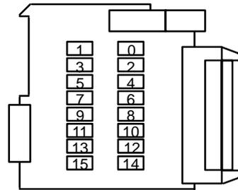
7. A Relay puller is provided inside the rear of the case when the Unit is delivered. Use the Relay puller to pull out the Relay as shown below. Insert a new Relay.
