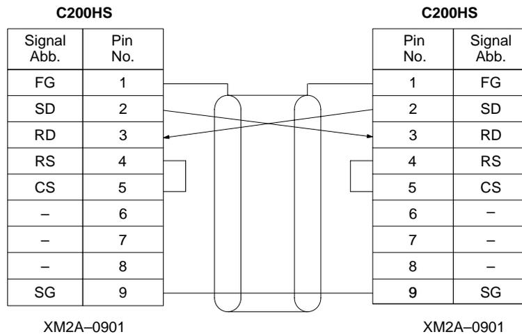
Ground the FG terminals of C200HS Units at a resistance of less than 100 Ω.
