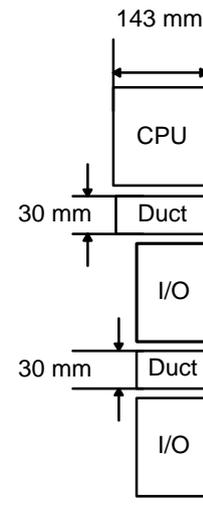
Each Rack must be mounted vertically, that is, with the printing on the front panels oriented as it would normally read. Racks may be directly mounted to any sturdy support meeting the environmental specifications.
