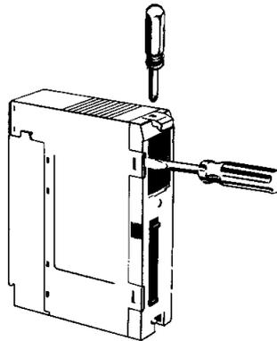
6. Pull out the printed circuit board. The Relays are placed on the PC boards of individual Units as shown in the figures below.
