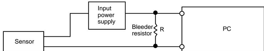
If the leakage current is less than 1.3 mA, there should be no problem. If the leakage current is greater than 1.3 mA, determine the resistance and power rating for the bleeder resistor using the following formulas.
