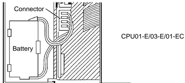
5. Replace the cover of the battery compartment.
