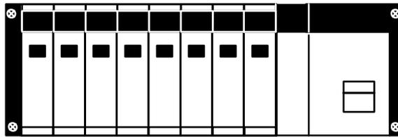
The figure above shows a total of eight I/O Units mounted to the Backplane. When using 16-point Output Units (models C200H-OC225/OD212/OD21A) mount them to a C200H-BC□□1-V1/V2 Backplane. If a Backplane other than this model is used, the Units will not operate properly.
