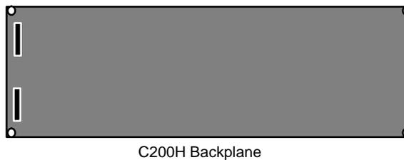
The Backplane is a simple device having two functions. The first is to provide physical support for the Units to be mounted to it. The second is to provide the connectors and electrical pathways necessary for connecting the Units mounted to it.
