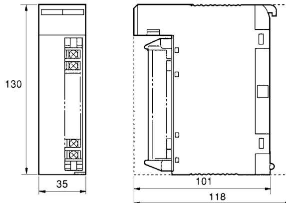
**19-terminal Terminal Block (B-shape I/O Units)**
