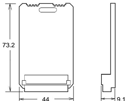
**C200H-PS221/PS221-C/PS211 I/O Power Supply Unit**
