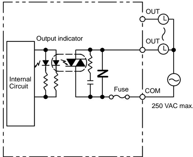
Fuse: 3 A 250 V (5.2-dia.x20) MQ4 (SOC)
