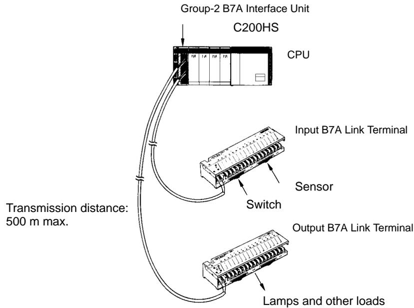
Group-2 B7A Interface Units can be mounted to a CPU Rack or an Expansion I/O Rack. They cannot be mounted to Slave Racks or to Racks controlled by any other CPUs.
